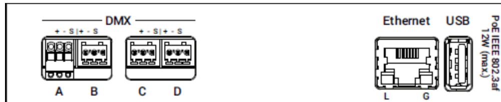
grandMA3 4Port Node DIN-Rail – rear panel
